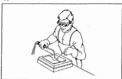
High temperatures may be obtained by the controlled burning of gases (oxy-acetylene welding),
