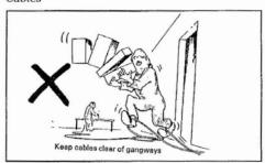
Keep cables clear of ladders, gangways, and doors. Do not allow traffic to pass over cables. Disconnect from power source before joining any cables. Never use damaged cables.
