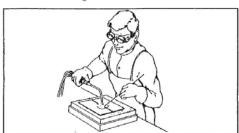
In leftward welding the flame is directed towards the unwelded part, and the filler rod, when used, is directed towards the welded part of the joint. With the blowpipe held in the right hand, welding proceeds from right to left; with the blowpipe held in the left hand, welding proceeds from left to right. In vertical welding the movement is upwards.
