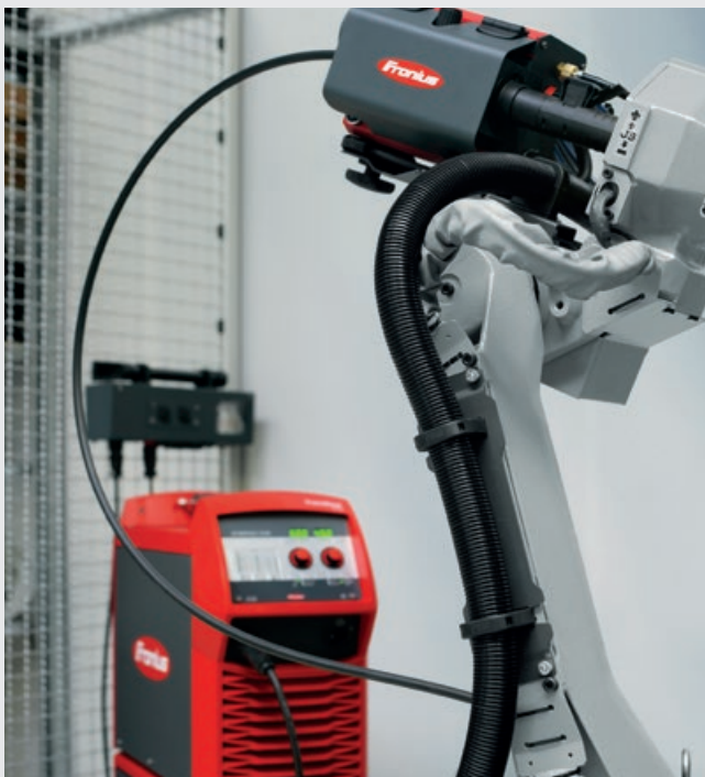
/ TransSteel Robotics system configuration.
